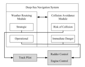
Figure 4: Autonomous navigation system architecture /7/
