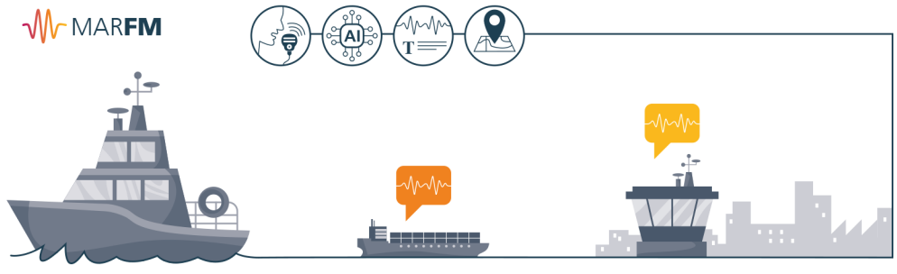
marFM® transcribes VHF voice radio into text using AI. © Fraunhofer CML
