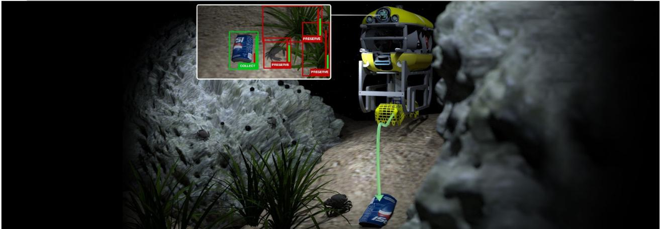
A robotic system intended to clean litter from the seafloor has passed its first real-life tests in waters near Dubrovnik, Croatia. The cleaning system, which works similarly to home robot vacuums, was able to see waste on the bottom of the sea and move towards it. A plastic bottle became the first official litter to be picked up from the seabed. This series of tests is a small step in humanity's goal of cost-effectively cleaning the seafloor, where more than 90% of the sea garbage is found.
