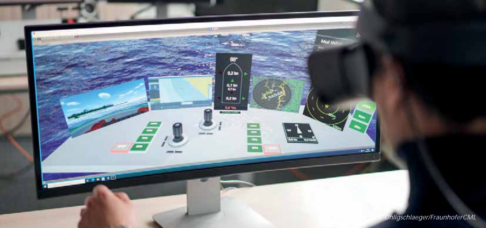
Figure 20: Steering a Tug remotely in mixed reality RoboTug project
