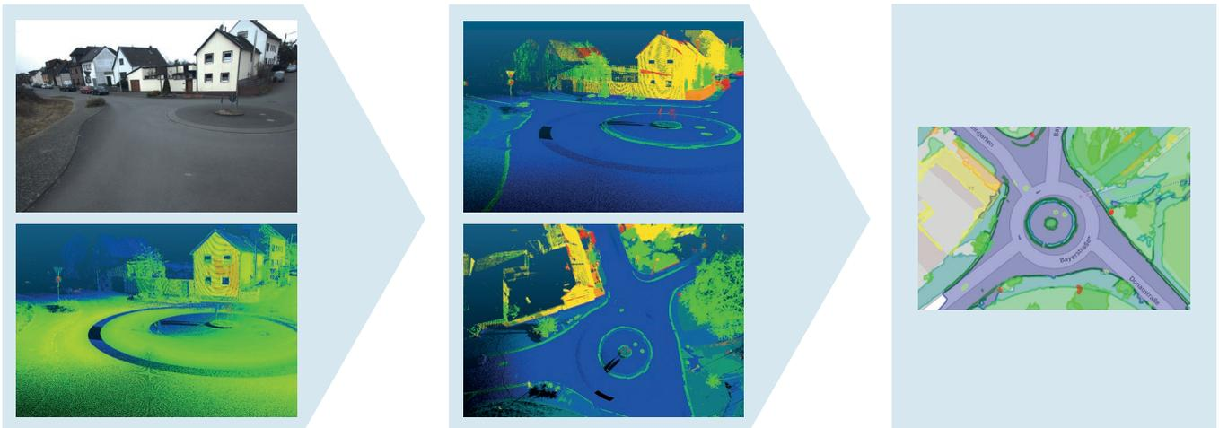
2D camera data (upper left) and 3D laser scanner data (lower left) depict the infrastructure quickly and efficiently. 3D-AI analyzes the data automatically using smart algorithms (Mid). Each color in the point cloud represents a singular class of objects. This data is then transferred to a digital planning map (right) for automated route planning. In addition to the categorized surfaces, this plan contains information on the position of the objects.
