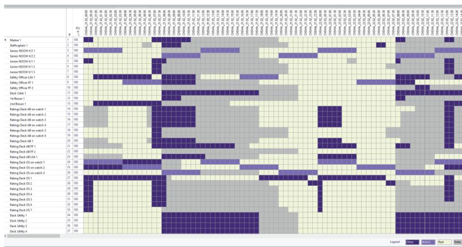
Image 3: SCEDAS® schedules the voyage dependent workload under the consideration of the crew's qualifications and rest hour regulations (watch displayed in light purple, other operational tasks dark purple, rest hours in beige and available time for maintenance in grey)
