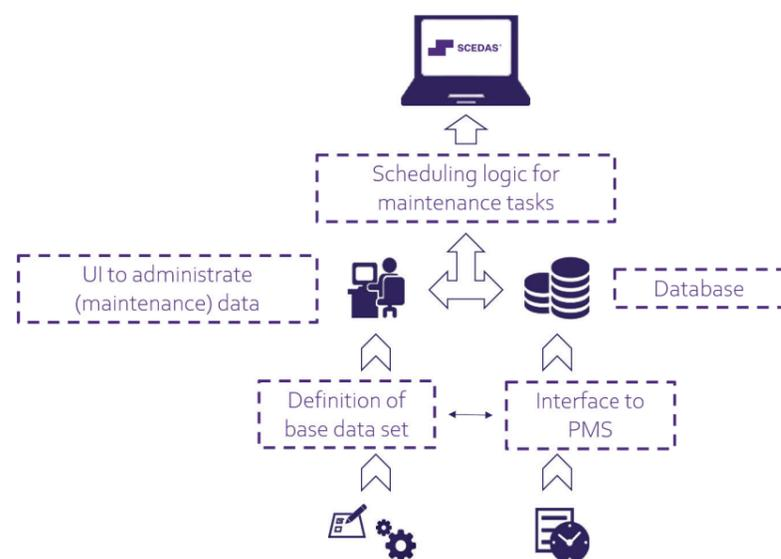
Image 5: implementation process of SCEDAS® with integrated maintenance scheduling
